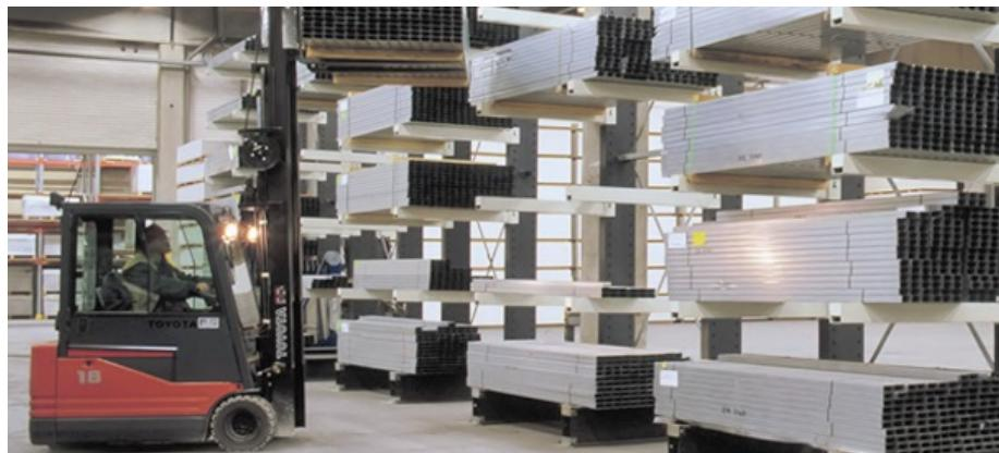
**Cantilever Racking, Pigeon-hole rack, Timber locker, A-rack and Rack for metal sheet etc are specially designed to store long goods and items of varying lengths.**
