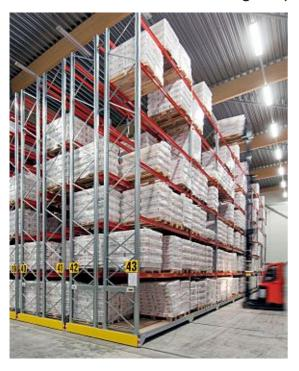
Mobile Pallet Racking can increase storage capacity in your Food and Drink warehouse considerably. P90 Pallet Racking is mounted on mobile bases that electronically move to create an access aisle for picking. By removing unnecessary aisles this enables you to store more stock on a smaller footprint.
