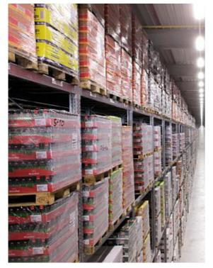
Even in a state of the art warehouse for Food and Drink, standard pallet racking is still the most common form of pallet storage. The versatility of this pallet racking system means this can be assembled in a single or double deep configuration, to fit your specific storage needs.
