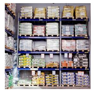
Pallet racking makes the ideal storage system for the storage of bulk goods on pallets. The versatility of pallet racking means that it can be used with a variety of shelving and display options, such as vertical storage, to provide bulk storage either alongside or above the main retail display area.
