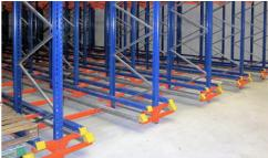
Saving space is important. Since the forklift trucks does not need to access the aisle, all channels can be fully utilised at all times providing extra storage space. The Pallet Shuttle System offer a high density and more effective storage method.
