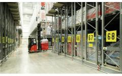
The electronically controlled MOVO heavy mobile racking systems run on in-ground rails and can carry bay loads of up to 24 tons at racking heights of up to 12 meters.
